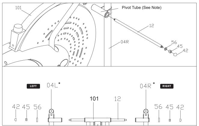
\* To avoid incorrect assembly, please use illustration above as reference and ensure #04L is installed on the LEFT side and #04R is installed on the RIGHT side.
