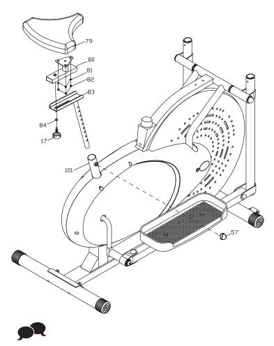
You may adjust the Seat Post (#83) to the height most comfortable for you after complete assembly. Please always check to ensure a hole has been fully engaged when you secure and tighten the Knob Bolt (#57).
