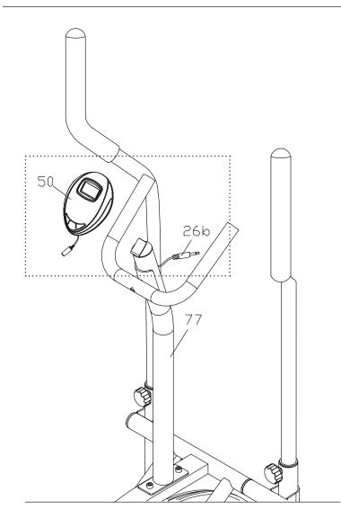
Connect the pin on the tip of the Sensor Wire **(#26b)** to the corresponding socket of the wire end on the Electronic Monitor **(#50)** as shown in diagram below.
