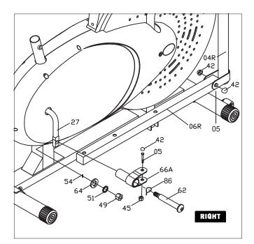
Remove Hex Bolts (#05) and Nylon Nuts (#45) that are pre-assembled on the Pedal Connection Joint (#66A) and set them aside as they will be used in a later process.
